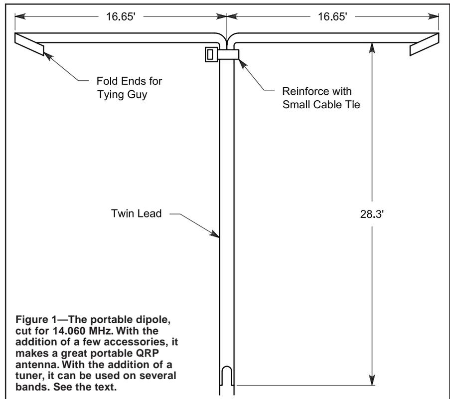
would normally compute using the formula  $984/f(\text{MHz})$ . I put a 50 ohm dummy load on one end of a 49 ft length of twin lead and used an MFJ 259B antenna analyzer to measure the resonant frequency, which was 8.10 MHz. The 2:1 SWR bandwidth measured 7.76 to 8.47 MHz, or about 4.4% from 8.10 MHz.
