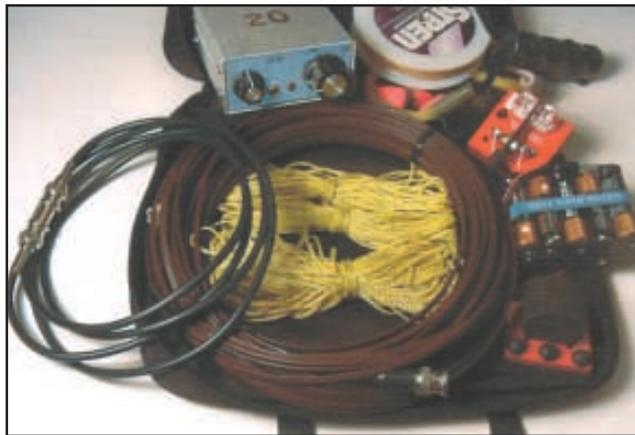
**Figure 2—The author's portable station, including twin-lead dipole, 20-meter Wilderness Radio SST transceiver and support line. It all fits in the 8"×10½"×2" Compaq notebook computer case.**
