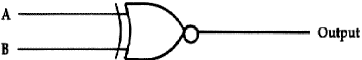
XNOR Gate (XOR with active low output)
